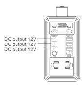
A. These three DC5521 (5.5mm in diameter) 12v ports offer max 8A output current and automatically
