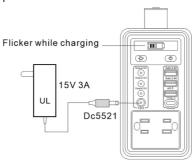
Plug the original adapter into the machine's AC input port and you will see the battery indicators on the screen blink.
