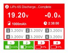
CH1 and CH2 charging completed (Green color) CH3 and CH4 discharging completed( Red color)
