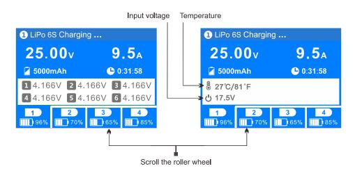
Rotating the roller wheel up or down during charging will switch the information displayed on the lower half of the LCD screen between cell voltage, cell IR and working parameters. Cell voltage and IR can only be displayed during the balance charging process.
