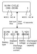
You can set up sequence on the left and the number of cycles on the right. Range of the cycle number is 1-5.
